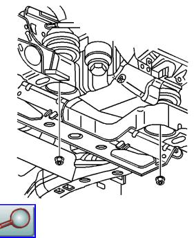
6. Install the lower engine mount bracket retaining nut.
