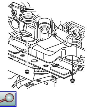
5. Remove lower engine mount bracket retaining nuts.
