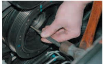
95. Install the new balancer bolt supplied.
