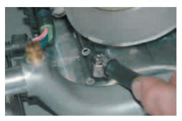
148. Route the 24" coolant line along the front of the supercharger manifold and under the Mass Air Flow meter (MAF). Use the supplied 1/4" hose connector and another #4 clamp to connect the coolant line to the vehicles coolant vent line using the original clamp.
