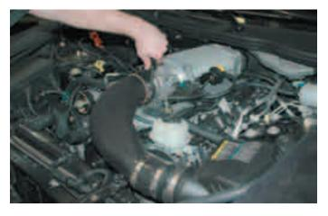
181. Here is the intercooler pump harness and components.
