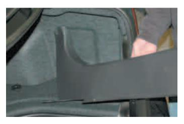
200. Pull the right interior panel out and push it forward to gain access behind it.
