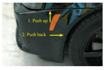
193. Re-install all the push reivets into their original locations in the fascia and wheel wells.
