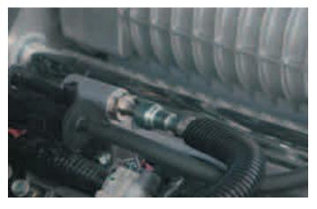
145. Re-install the fuel line retaining clip.
