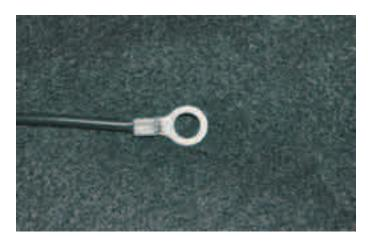
204. Remove the ground connection bolt with a 10mm socket wrench and install the module black ground wire on it. Re-install the bolt and tighten securely.
