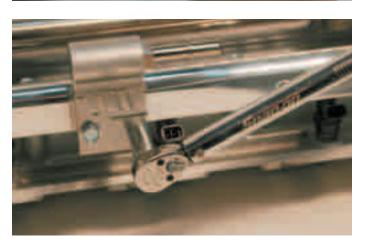
112. Remove the Manifold Absolute Pressure (MAP) sensor from the stock intake manifold by tilting the sensor forward and lifting it free. Ensure that the orange rubber seal is not missing or damaged as it and the sensor will be re-used.
