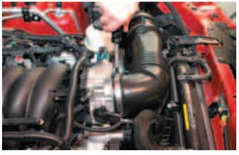
41. Remove the air tube completely, as it will not be reused.
