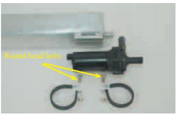
161. Install two of the round head bolts into the slotted rail on the front of the reservoir as shown. Note that the square portion of the bolt shaft must be aligned with the sides of the channel.
