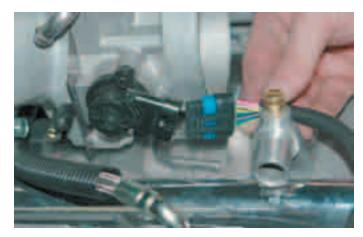
126. Install the ETC connector onto the throttle body.
