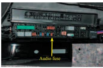
3. Pull back the carpet where it meets the seat base on the right (passenger) side to expose the other fuse CENTER. Remove the fuse center cover and examine the legend printed inside the cover to locate the fuse marked "Fuel Pump Mtr".
