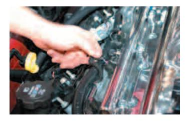
124. Install the TPS extention harness onto the harness connector.
