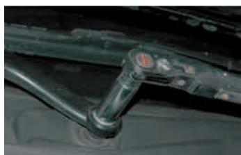
27. On the top of the strut towers remove the two bolts on each side that secure the strut tower brace with a 18mm socket wrench.
