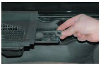
23. Re-install the wiper assembly into place. Note that the mounting bolt will pass through the spacer washer installed in the previous step.
