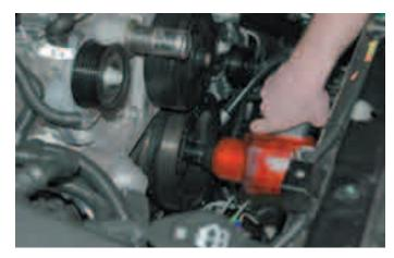
86. Install the drill guide and bolt into the stock location. Note that the smaller diameter end of the guide goes towards the balancer.
