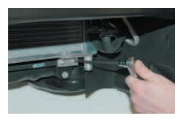
158. Remove the lower right A/C condensor mounting bolt with a 10mm socket wrench. Install the two reservoir brackets using the A/C mounting bolt and a new supplied bolt in the center attachment point on the radiator tank.
