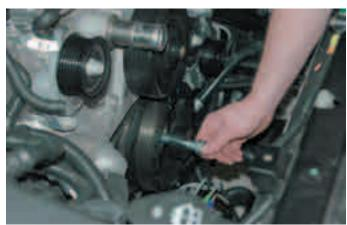
87. Torque the guide bolt to 60 ft-lbs with a torque wrench and 24mm socket.
