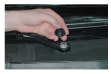
12. Remove the wiper arm attachment nuts with a 15mm socket wrench.
