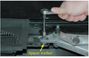
25. Replace the wiper aprons, mounting screws and weather strip into their original locations.
