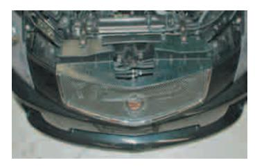
192. Line up the lock bolt heads with the "keyhole" slots in the bottom edge of the fender. Push up on the fascia and then back to re-attach the fascia to the fenders. Rotate the steering wheel to move the road wheels inward on each side to gain acess to the lock bolt nuts through the wheel well. Take care to ensure the fascia lines up correctly and tighten the lock bolt nuts securely.
