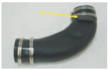
179. Install the air tube assembly by pushing it against the MAF and then sliding the hose and clamps on to it.
