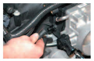
50. Disconnect the vacuum brake booster valve from its mounting grommet on the booster.
