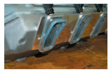
116. Remove the tape from the port surfaces and using silicone spray or soapy water apply a light film to allow the port gaskets to slide on the surfaces. Do not use any petroluem based lubricants as these will damage the port gaskets.
