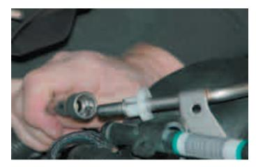
58. Remove the two coolant lines attached to the bottom of the throttle body.
