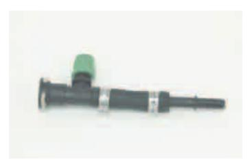
142. Install the new EVAP hose onto the rear barb of the purge solenoid and into the firewall connector. Next connect one end of a 12" length of 3/8" hose to the front barb of the purge solenoid.
