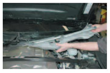
21. From the top surface of the left wiper arm lever, measure down 3/8"(10mm) and scribe a line across the lever. Using a suitable grinder or saw remove all the material above this line.
