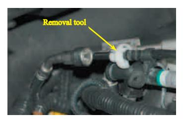
54. Remove the Purge solenoid and EVAP line by pulling the solenoid free from its mounting location on the left side of the intake manifold.
