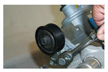
76. Install the new tensioner assembly in place of the stock unit with the supplied bolts and torque them to 40 ft-lbs.
