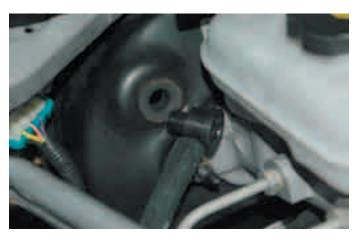
136. On the driver (left) side of the engine connect the brake hose to the large barb on the inlet manifold. Route the brake hose along the side of the engine and behind the supercharger to the brake booster.
