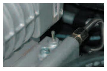
213. Using the presure switch and the small vacuum hose supplied attach the pressure switch to the vacuum nipple on the manifold. Route the switch forward to lay beside the wiring harness and secure it there with the cable ties supplied. Connect the red and black wire connectors from the fuel pump booster cable to either pressure switch spade connection.
