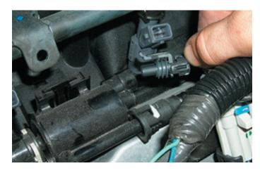
52. Press the white release trigger on the Evaporative emission (Evap) pipe connector to remove it from the barb on the intake manifold. Disconnect the other end of the Evap pipe from the purge solenoid.
