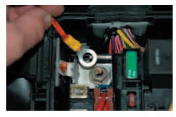
188. Place the relay into the rear corner of the Fuse/Relay center. Using a sharp knife, cut away at the top of the harness boot to allow the ground and pump wire from the relay to pass from the inside to the engine compartment.
