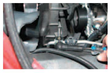
82. Disconnect the radiator fan electrical connections on each fan by squeezing the connectors and pulling them free.
