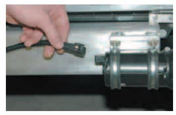
190. Re-install the front fascia by first re-connection the four electrical connectors on the inside of the fascia.
