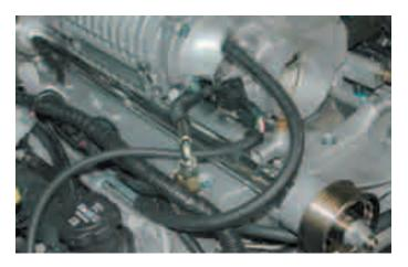
130. At the rear of the driver side valve cover, remove the rubber cap covering the PCV barb.
