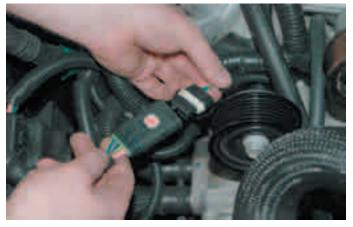
125. Install the TPS extention connector onto the throttle body connection.
