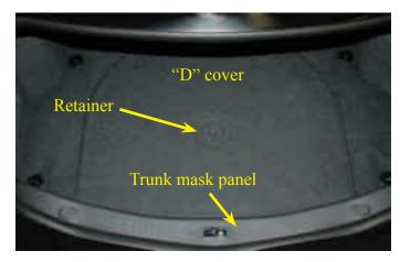
195. Remove the four retainer buttons that secure the trunk mask panel to the rear of the trunk by unscrewing them. There is one button on the floor and one on the wall on each side
