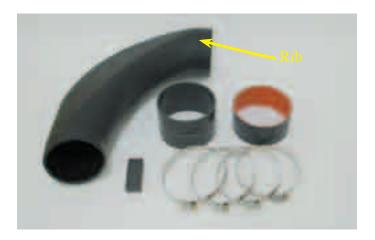
178. Assemble the air tube assembly by sliding the hoses all the way onto the air tube and then place the #60 clamps in position. Note that the shorter of the two hoses will go on the end of the tube with the raised "Rib". Do not tighten the clamps at this time. Peel the paper backing from the rubber pad supplied and attach the pad to the underside of the air tube in the position shown.
