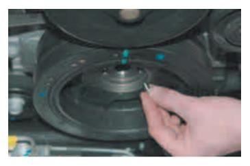
94. Use a small hammer and a drift to tap the dowel pins in as far as they will go into the balancer.
