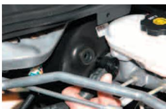
51. Above the driver side (right) valve cover, disconnect the Evaporative Purge Solenoid (EVAP) electrical connector.
