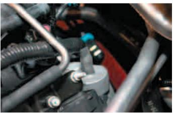
131. Assemble the new PCV outlet hose by cutting a 43" length and a 2" length of the 3/8" hose. Attach one end of each hose to the 90 degree elbow fitting.
