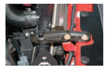
78. Remove the Air conditioning (A/C) condensor from the radiator by removing the four bolts along the top and bottom radiator tanks with a 10mm socket wrench.
