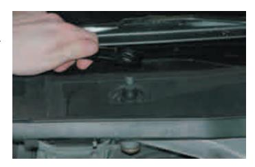
14. Remove the rubber weather strip from the front edge of the wiper arm apron.
