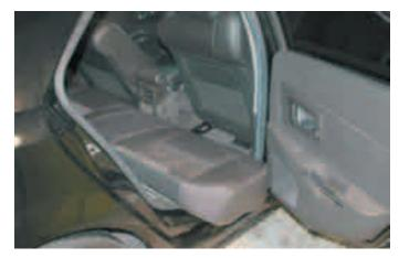
2. Once the seat cushion has been removed pull back the carpet where it meets the seat base on the left (driver) side to expose the fuse center. Remove the fuse center cover and examine the legend printed inside the cover to locate the fuse marked "Audio". Remove the 10 amp "Audio" fuse so the vehicles PCM (engine management computer) can be re-programed safely. THIS FUSE MUST BE REMOVED BEFORE REPROGRAMING!
