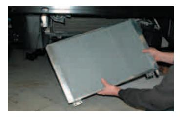
157. Bolt the heat exchanger into place using the supplied Allen bolts and a 4mm Allen socket wrench.
