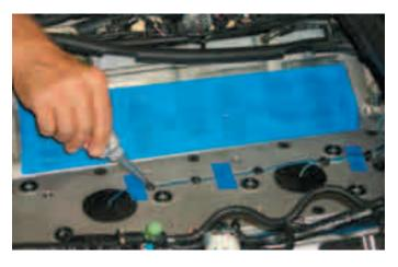
72. Remove the two coolant vent pipe bolts with a 10mm socket wrench.
