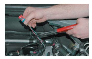
102. Using the new lengths of color coded wire and crimps connectors supplied to extend the purge solenoid connector wires. Strip about 1/4" of insulation from the ends of all the wires, then crimp the connectors on. Using a heat gun or blow dryer set on "High" shrink the insulation on the crimp connectors so that it contracts around the wires completely. You must shrink the insulation, as crimping the connections alone is not enough to secure them!
