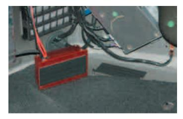
202. Here is the module mounted in location. The chassis electrical ground connection on the wall above the module. This is where the module ground connection will be connected.
