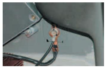
205. Locate the large branch of the wiring harness running down the wheel well. Carefully cut the tape and locate the large **GREY WIRE**. Pull the large grey wire out of the bundle, this is where the booster connections will be made.
