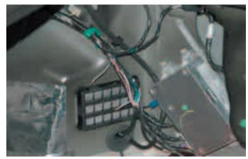
207. Using the crimp connectors supplied, connect the large **RED** wire with the in-line fuse to the **Upper grey wire.** Connect the remaining large **Red** wire to the lower grey wire that runs to the fuel pump.
