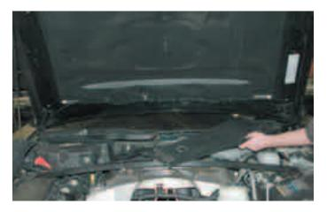
18. Located on the bottom of the wiper assembly is the wiper motor electrical connector. Disconnect the connector from the motor.
