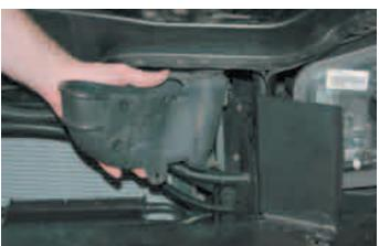
167. To remove the boot, drill out the two mounting rivets at the front of the boot.
