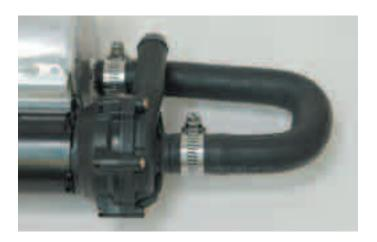
174. Attach the "L" shapped hose to the pump outlet barb and the heat exchanger inlet barb using two #10 clamps supplied.
