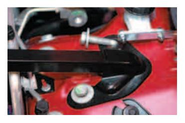
28. Remove the strut tower completely, as it cannot be reused with the supercharger. Replace the bolts into their original holes and torque them to 83 ft-lbs. While the strut tower brace is not completely necessary, a replacement to fit around the supercharger system is available from Lund Cadillac Performance Division Inc. Contact them at 1-602-375-4383
