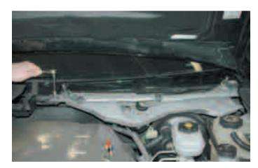
20. Remove the wiper assembly complete from the vehicle
