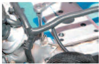
75. Remove the stock belt tensioner assembly by removing the two mounting bolts with a 15mm socket wrench.
