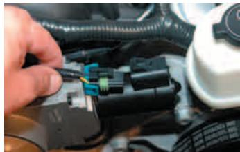
43. Disconnect the Throttle Position Sensor (TPS) connector on the right (passenger) side of the throttle body.
