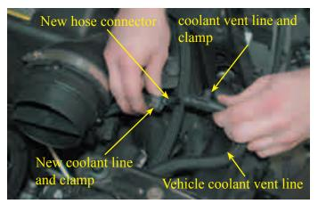
149. Install one end of the 20" length of 1/4" heater hose on the coolant vent pipe barb. Secure the hose with a #4 clamp supplied.
