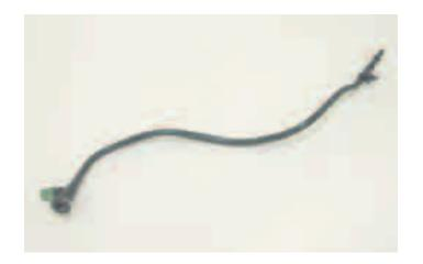
138. Using a sharp knife, carefully cut the plastic pipe so that the end fittings can be reused.
