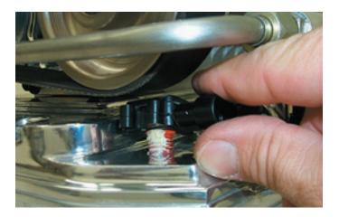
114. Install the MAP sensor in its new location using the supplied bracket and the button head Allen screw with a 4mm Allen wrench.
