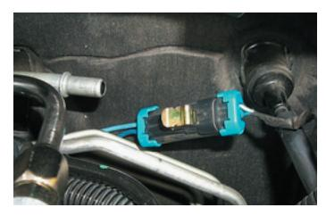
122. Install the ignition coil pack connectors on both sides of the engine.
