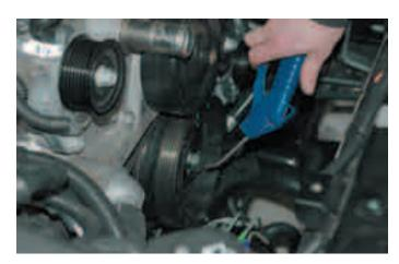
92. Remove the drill guide and bolt from the end of the crankshaft.
