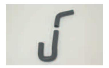
170. Cut approximately 3" off the short leg of the large "L" hose supplied as shown.
