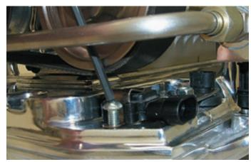
115. Install the eight intake port gaskets into the recesses on the manifold faces. Ensure that the tab on the gasket aligns with the slot on the manifold face. Inspect the manifold ports for any dirt or foreign matter.
