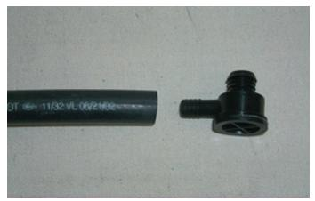
135. Install the new check valve and hose onto the brake vacuum booster.
