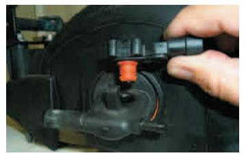
113. Apply a small amout of the grease supplied to the MAP sensor seal and install the sensor in its new location at the right rear of the supercharger manifold.
