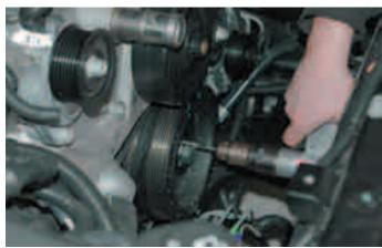
91. Use some compressed air to remove any material from the holes.
