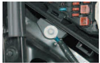
187. Connect the Red positive (+) wire with the ring terminal to the main power connection on the Fuse/Relay Center.
