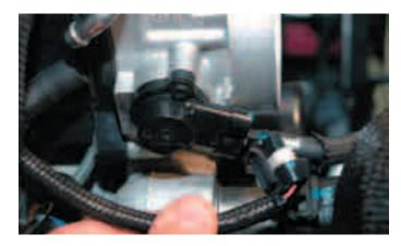
44. Disconnect the eight injector electrical connectors.
