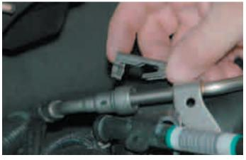
57. Disconnect the fuel pipe from the large quick-release fitting using the supplied removal tool. Snap the tool on the pipe and push it into the quick release fitting to release the pipe.
