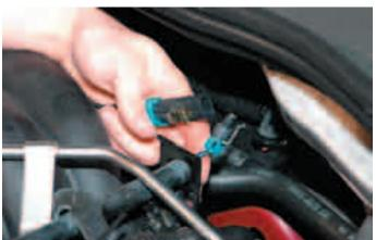
47. Disconnect the Manifold Absolute Pressure sensor connector at the rear of the intake manifold.
