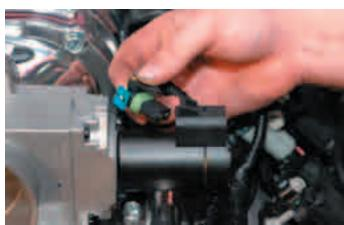
127. Install the purge solenoid onto the new bracket and then install the EVAP electrical connector.
