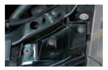
194. Re-install the lower front splash panel with its push rivets.
