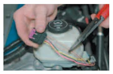
98. Using the new IAT harness, lengths of white wire and crimps connectors supplied, Install the IAT connector and extention wires to the two ends of the brown wires leading to the computer. It does not matter which white wire connects to either brown wire. The two wires from the MAF connector will no longer be used.
