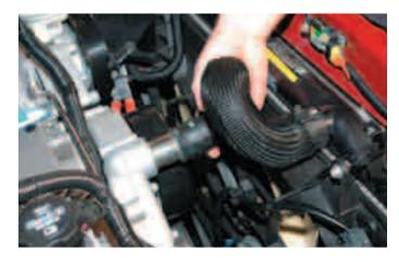
80. Disconnect the radiator vent hose from the top tank by squeezing the hose clamp with a pair of pliers and pulling the hose off.
