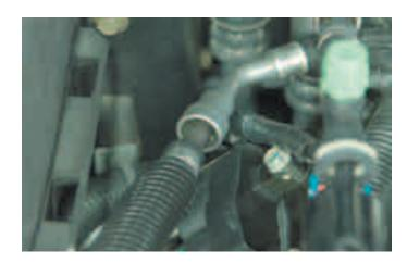
144. Connect the remaining end of the fuel line extention to the fuel manifold connector
