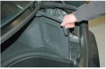
201. The fuel pump booster will mount on the trunk floorusing the supplied Velcro strips supplied. Peel the backing off the two Velcro strips and apply it to the botton of the module and to the trunk floor near the two studs on the floor.
